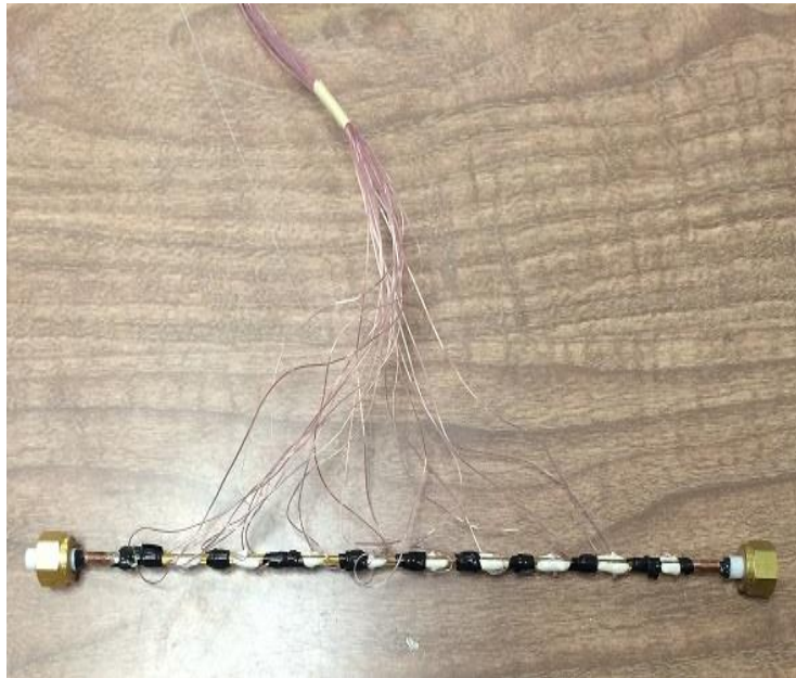
Figure 3.12 Square test section with thermocouples tips cemented axially along the surface using Omega bond cement.
