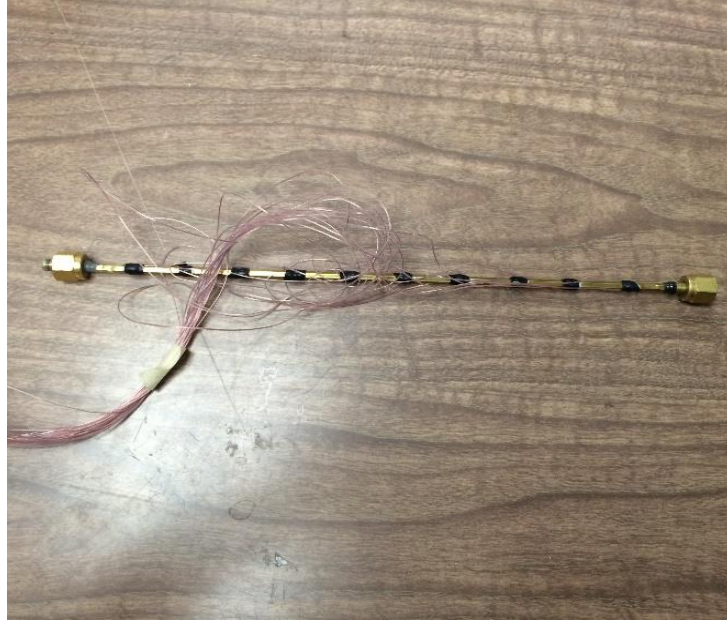
Figure 3.13 Hexagonal test section with thermocouples tips cemented axially along the surface and two copper strips at the end for supplying DC power.
