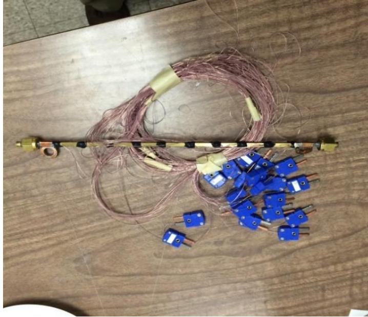
Figure 3.11 Rectangular test section with thermocouples tips cemented axially along the surface and two copper strips at the end for supplying DC power.
